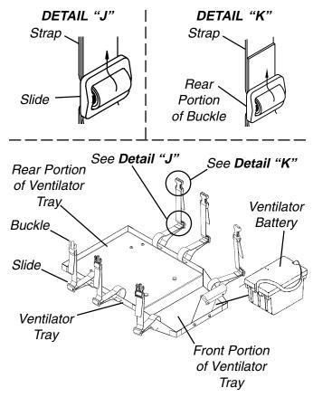
FIGURE 6 - USING THE VENTILATOR TRAY
